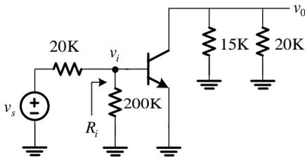
$$R_i = 200\text{K} // 5.47\text{K} = 5.324\text{k}\Omega$$
