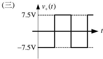
$$v_+(t) = \frac{R_2}{R_1 + R_2} v_0(t) = \frac{1}{2} v_0(t)$$
